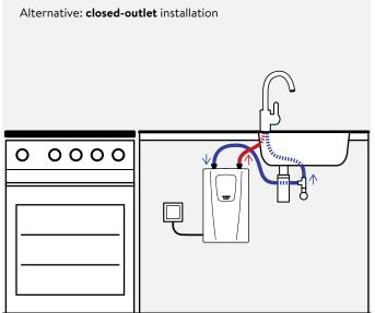
Electrical connection with **load shedding switch LAB** at only one existing 400 Volt cooker terminal outlet box, if no separate outlet is available for the instant water heater.
