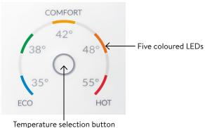
Touch the button to select the next temperature setting (35°C, 38°C, 42°C, 48°C or 55°C).
