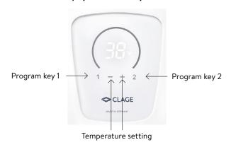
The DCX12 Next L is operated via a LED display with sensor keys. The two programming keys are preset to 38 °C and 42 °C and can be individually adjusted. Unit parameters can be read out and set via a service menu.
