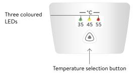
Touch button controls for temperature selection. Press the button to select the next temperature setting (35  $^\circ$ C, 45  $^\circ$ C or 55  $^\circ$ C).
