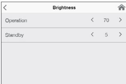
**Brightness:** Reduce the display brightness e.g. to save energy. The brightness can be set separately for operation screen and standby mode.
