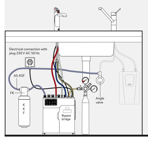
Example installation with **KKF in the cold water inlet** of a Zip HydroTap® G5 BCS for softening the hot water and simultaneously filtering the cold water.
