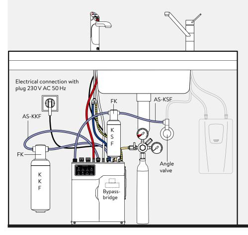
Example installation with **KSF in the cold water inlet** and additionally with a **KKF in the hot water bypass** of a Zip HydroTap® G5 BCS.
