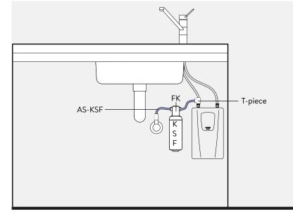
Example installation with KSF in the cold water connection of a pressurised tap.
