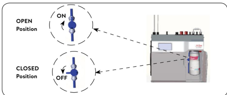
**Note:** Run at least 10 ltrs of water through to flush the filter of any excess black carbon particles (this is normal).
